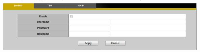
**DynDNS** – Enable the DynDNS to allow the camera to have a fixed host and domain name. Refer to the DynDNS website (www.dyndns.com) to apply for a dynamic domain account. When an account has been created, enter the username, password and hostname. Click **Apply** to apply settings or **Cancel** to cancel changes.
