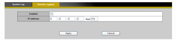
The user can configure the camera to send the system log file to a remote server as a log backup.
