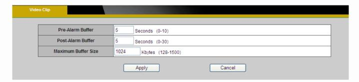
This function is used to determine when video clips will be recorded and stored after an event is triggered.
