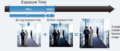
A single high-contrast frame is created by combining the two frames using an advanced image signal processor.
