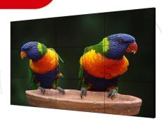
The DS-D2046NL-C LCD display uses an industry-level ultra-narrow bezel design, which enables a bezel width of 3.5 mm between neighboring displays. The adopted direct-lit LED backlighting technology helps achieve ultra-high and uniform brightness of 500 cd/m² without boundary shadows. The display has abundant interfaces for video inputs, such as DVI, VGA, and HDMI.
