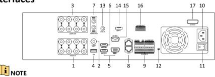
The rear panel of DS-9016HUHI-K8 provides 16 video input interfaces.
