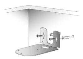
2.Fix the camera to the bracket with the two supplied screws (typeA).
