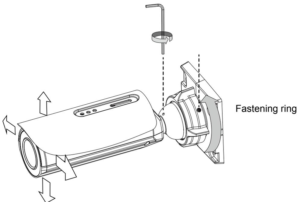
3. Secure the Network Camera to a wall or ceiling.
