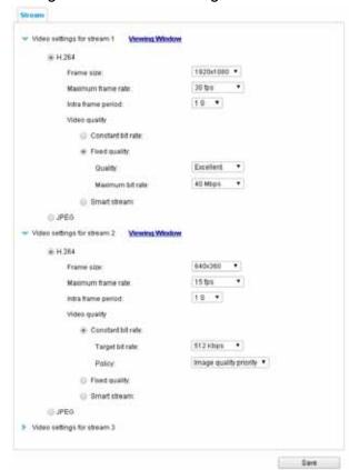
This Network Camera offers real-time H.264 and MJPEG compression standards (Dual Codec) for real-time viewing. If the H.264 mode is selected, the video is streamed via RTSP protocol. There are several parameters through which you can adjust the video performance:
