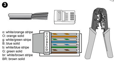
You will need an RJ45 crimping tool to attach the Ethernet wires to a connector. When done, connect the cable to the camera's Ethernet RJ45 socket.
