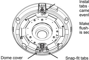
Install the plastic dome cover by aligning the snap-fit tabs on the dome cover with the slotted tabs on the camera base. Install the dome cover by pressing it evenly to the camera base.
