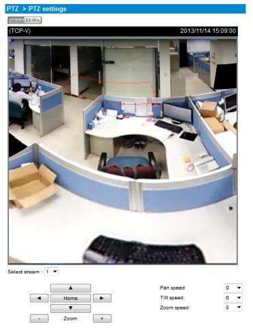
In this window, functional items related to the preset positions have been cancelled. This window is now used for changing the field of view when the Local dewarp function is applied to a video stream.
