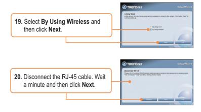
**Note:** The TV-IP501W will not work wirelessly until you disconnect the Ethernet cable from the back of the camera
