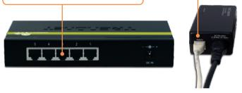
3. Connect a CAT-5e/6 cable from the TV-IP501P to the TPE-111GI's **DATA OUT** port.
