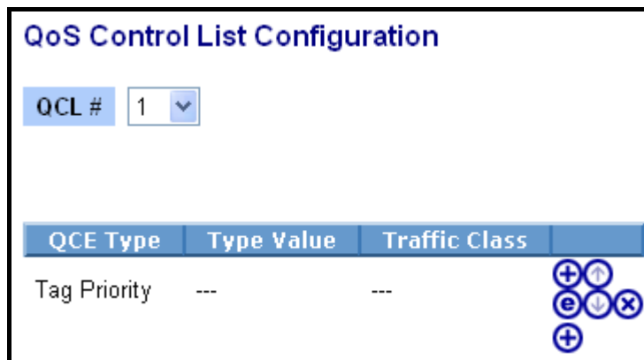
Fig. 3-62 Set up VLAN Tag Priority Mapping Finish
