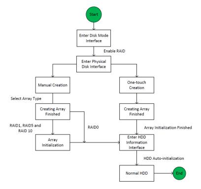
Figure 11.1 RAID Working Flow
