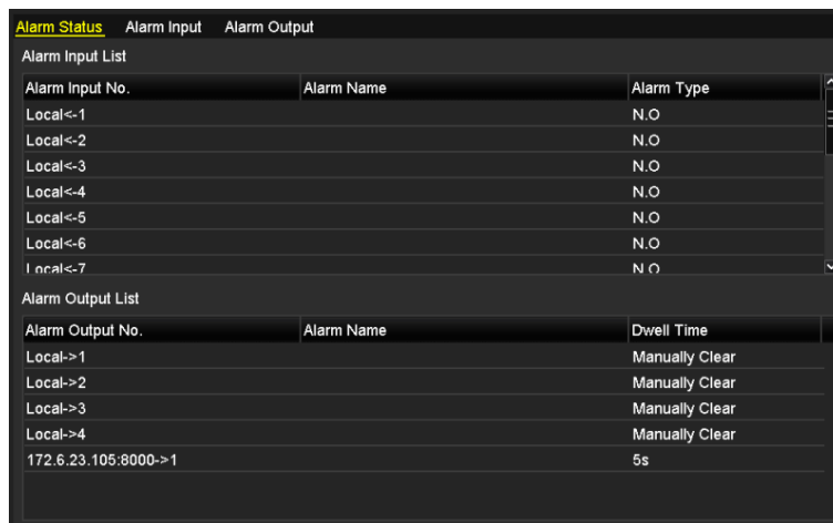
Figure 8. 4 Alarm Status Interface of System Configuration
