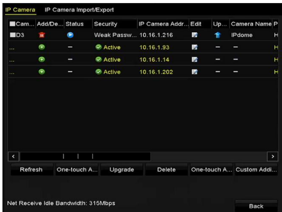
Figure 2. 19 Successfully Added IP Cameras
