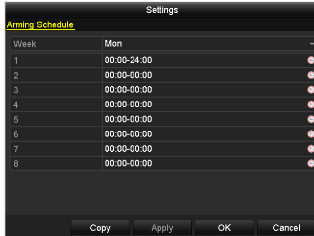
Figure 8. 20 Set Arming Schedule of Alarm Output
