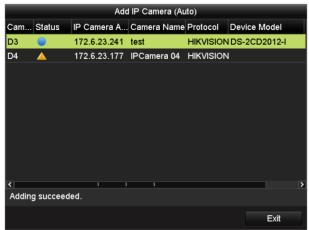
Figure 2. 13 Auto Adding IP camera Interface
