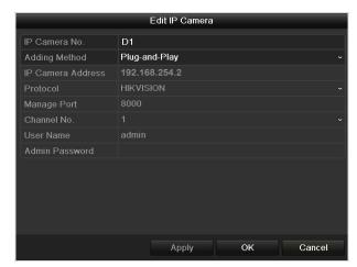
Figure 2. 25 Edit IP Camera Interface - Plug-and-Play
