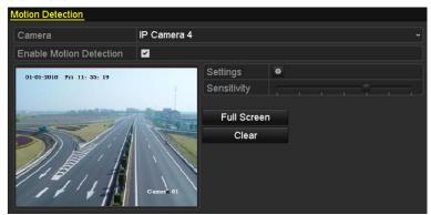
Figure 8. 1 Motion Detection Setup Interface
