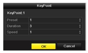
Figure 4. 6 Key Point Configuration
