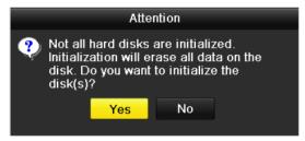
Figure 10. 1 Message Box of Uninitialized HDD
