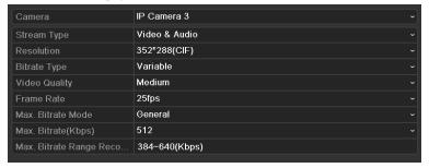
Figure 5. 3 Sub-stream Parameters
