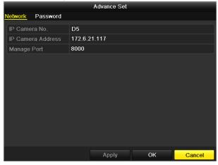
Figure 2. 20 Network Configuration of the Camera
