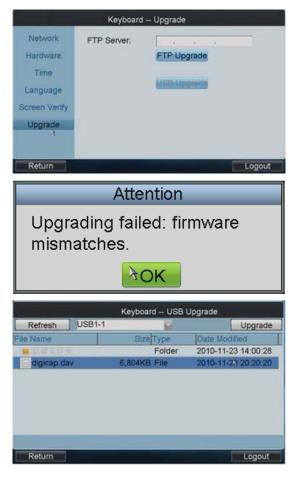
If the upgrading is failed, the corresponding error message box will pop up.
