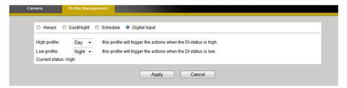
**Digital Inputs (\*)** (Only available with models with a DI terminal)- Select Digital Input to have the profile management controlled by an external sensor. Select profiles from the drop down menu. Profiles will change according to different trigger voltage levels. Click **Apply** to apply settings or **Cancel** to cancel changes.
