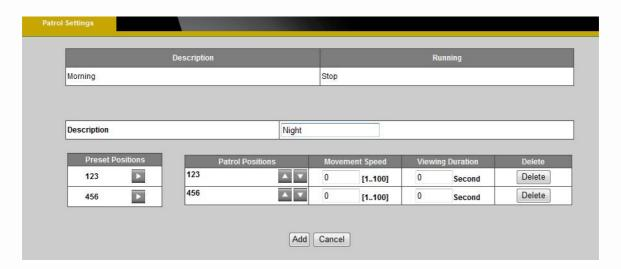
The camera can be set to patrol a group of preset points. For each patrol group, the user can configure the preset point order, movement speed, and viewing duration.
