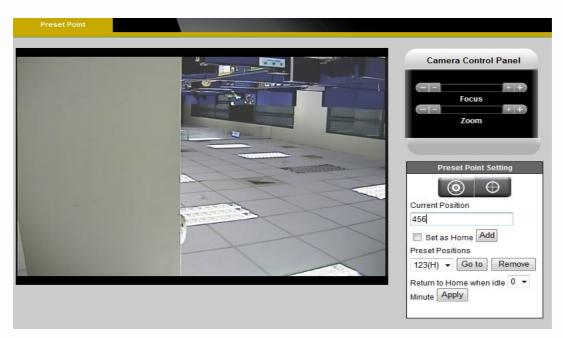
A preset position is a pre-defined camera view that can be used to quickly move the camera view to a specific location. To create a preset position:
