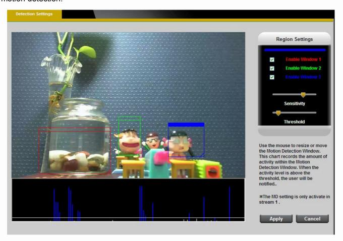
**Detection Setting –** Use this setting to enable and define the motion detection windows. The user can defined up to three areas on the live view window for motion detection.
