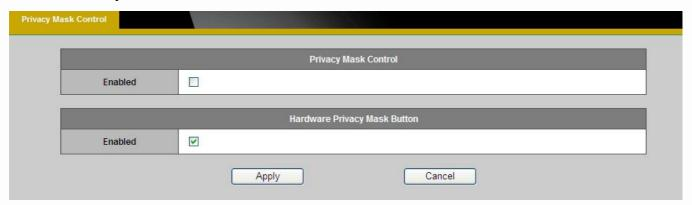
**Privacy Mask Control** – Enable the Privacy Mask control to remotely mask the camera's live view.
