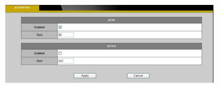
**HTTP** – (HyperText Transfer Protocol) - This protocol allows for TCP protocol quality without having to open specific ports for streaming. Users inside a firewall can utilize this protocol to allow streaming data through.
