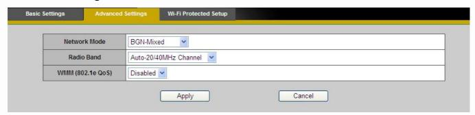
**Network Mode** - From the drop-down menu, select the wireless standards running on the network.
