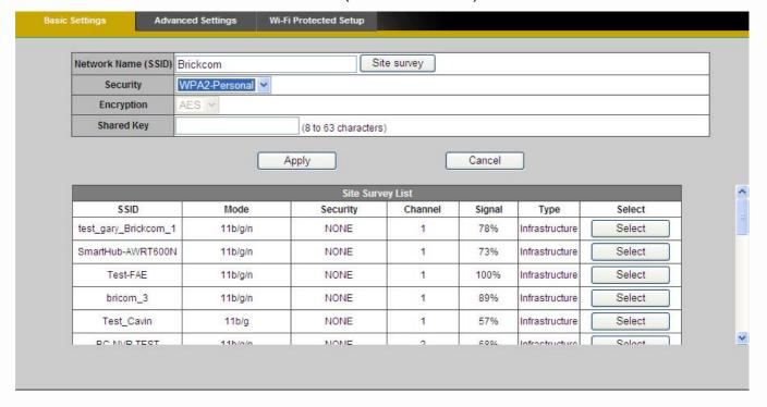
Encryption - WPA2 supports AES encryption method with dynamic encryption keys.
