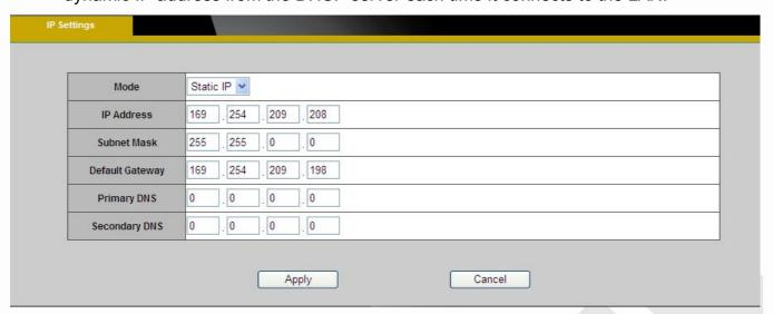
Static IP - Select this option to manually assign a static IP address to the camera. Enter
