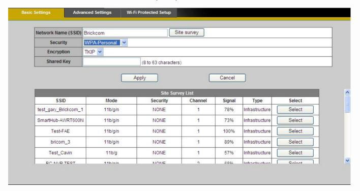
**Encryption -** Supports two encryption methods with dynamic encryption keys: Temporal Key Integrity Protocol (TKIP) and Advanced Encryption Standard (AES). Select the algorithm type from the drop down menu: TKIP or AES. The default is TKIP.
