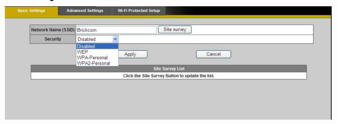
Network Name (SSID) - The Service Set Identifier (SSID) is the network name used to identify the wireless signal emitted from a wireless camera. It is case-sensitive and can be up to 32 characters long.
