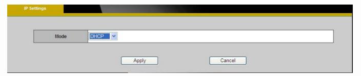
1. **DHCP** –If this option is selected, the camera will automatically obtain an available dynamic IP address from the DHCP server each time it connects to the LAN.
