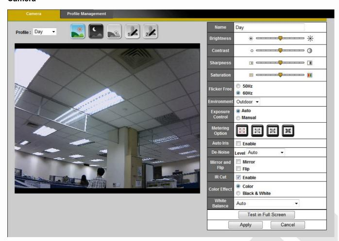
**Profile –** Up to five profiles can be created for different lighting environments. Day and night are default profiles and users can create up to three additional profiles. Select a profile from the drop-down menu or select different icons to change profile settings.
