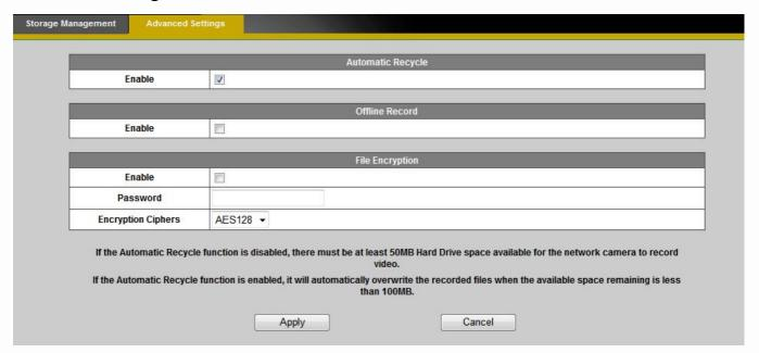
**Automatic Recycle (\*)** – Enable to automatically overwrite older files when the available space remaining on the Micro-SD/SDHC card is less than 100MB. If the Automatic Recycle function is disabled, there must be at least 50MB hard drive space available for the camera to be able to record video files.
