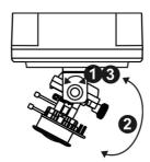
iii. Release the video adjustment screw and then adjust the lens direction. After completion, tighten the video adjustment screw.
