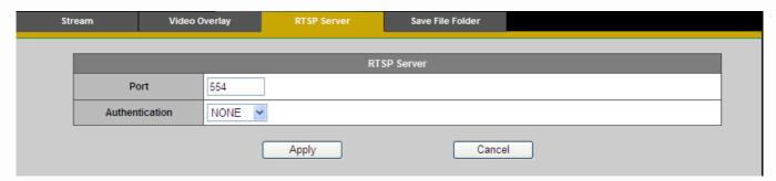
To utilize RTSP authentication, the user must first set a password for the camera. RTSP (Real-Time Streaming Protocol) controls the delivery of streaming media. By default the port number is set to 554.
