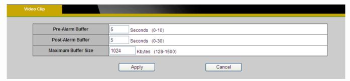
This function is used to determine when video clips will be recorded and stored after an event is triggered.
