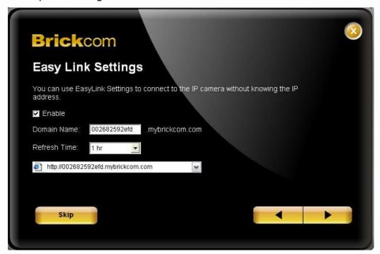
EasyLink™ is a unique Brickcom function which allows users to assign a unique domain name to their network camera's IP address. There is no need to configure the router to open up ports or remember hard-to-memorize IP addresses. When this feature is enabled, users can log onto [uniquedomainname].mybrickcom.com to view the camera's web GUI and live view.
