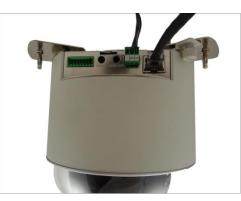
**NOTE:** The cables may be routed along the ceiling if the camera is installed on a hard ceiling. Or, the cables may pass through a hole on the ceiling if the camera is installed on a dropped ceiling.
