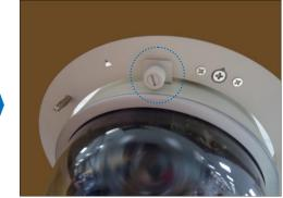
3. Tighten the screw on the fixing bracket to fix the camera position. This is to avoid accidental camera movement as the camera performs PTZ functions.
