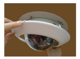
2. Push to firmly secure the cover ring latches.
