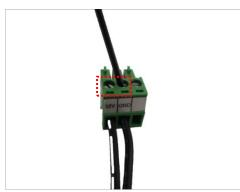
5. Set the prepared power adaptor for connection later. Below is an example of a power adaptor with an attached terminal block.
