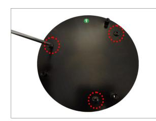
2. Secure the base plate to the ceiling or wall using the supplied screws.
