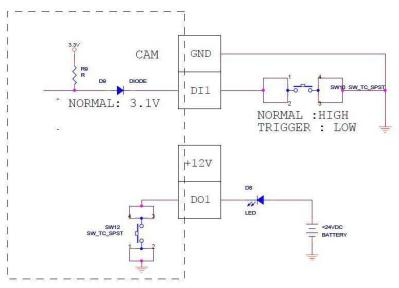
Consequently, to connect a second DI or DO device, wire the connection to Pins 5 to 8.
