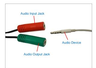
**Note:** Make sure that the connected audio input device has a built-in amplifier. Connecting an ordinary microphone will dwarf sounds and will result in inaudible recording.
