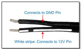
3. Connect the wire with the white stripe to the **12V** pin and the other to the **GND** pin.
