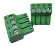
Map the pins according to one of the pin combinations on the table below. Loosen the screw and insert the wire through the pin slot on the terminal block, then tighten the screw to secure the wire. Connect the terminal block(2) to the corresponding cable connector(s).
