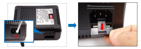
2. Remove the main fuse from its bay and pull to retrieve the replacement fuse.
