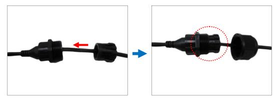
9. Attach the clamping nut to the cable gland body. Make sure the clamping nut is tightly secured and the rubber is squeezed in to avoid water leakage.
