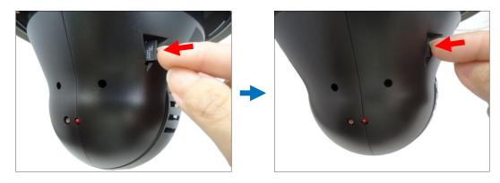
5. Align the screw holes and tightly secure the screws using the bundled hex screwdriver.
