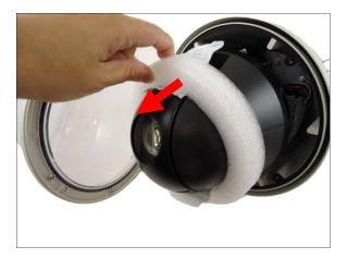
4. For I910 model, if a memory card will be used for local recording, insert the memory card at this point.
