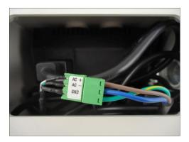
4. Install a female power socket (not included) inside the junction box to plug the cord and power up the camera.
