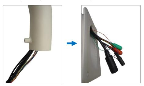
CAUTION: The camera itself is waterproof, however take note that the cable connections are not. If the cable connections will be exposed outdoors, make sure to shield or adapt proper waterproofing methods. See Step 3: Waterproof the Cable Connections on page 20.
