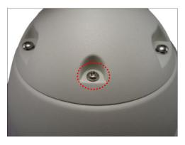
2. Insert the screw through the smaller end of the safety wire strap and attach it to the camera.
