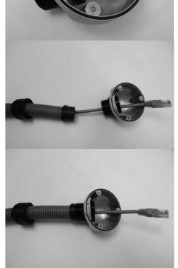
6. Pull the network cable through the back side cover of the camera.
