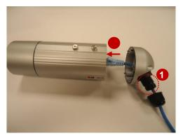
5. Assemble the Seal and Claw, and then Insert the network cable to RJ-45 PoE connector.
