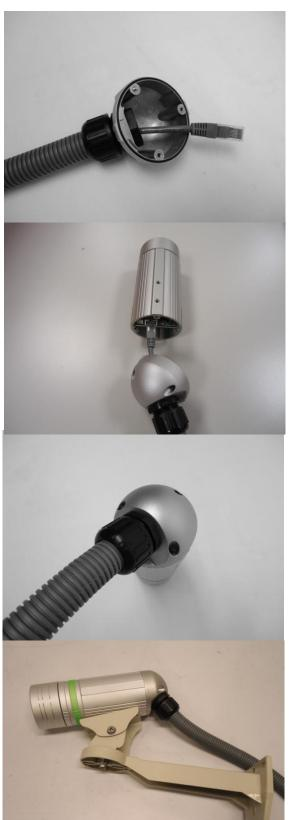
8. Tighten the domed sealing nut.
