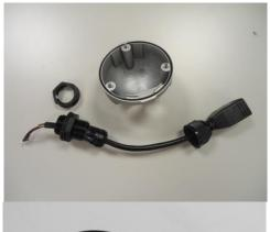
3. Remove the bundled network cable and connector from back side cover of the camera.
