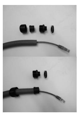
Disassemble the conduit gland as shown on the photo.
