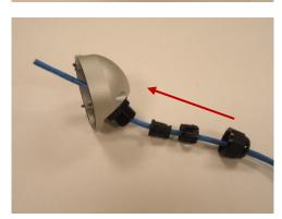
4.Pull the new network cable through Sealing Nut, Claw, Seal and cable gland on the back side cover of camera sequentially.
