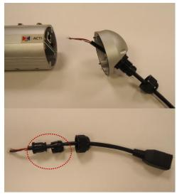
1. Open the back side cover from camera, and remove the network cable, and loosen the sealing nut to release the network cable from camera.
