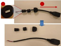
3. Squeeze the seal and then pull out the bundled network cable.
