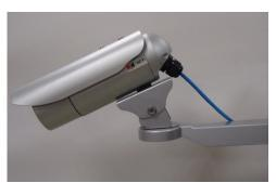
8. Finally, the bullet camera is now properly mounted with waterproof cabling and is ready to attach to the proper outdoor bracket.
