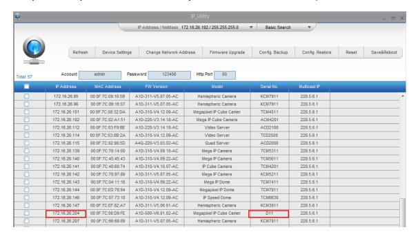
You can quickly notice the **D11** model in the list. Click on the IP address to automatically launch the default browser of the PC with the IP address of the target camera filled in the address bar of the browser already.
