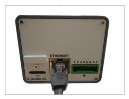
If necessary, connect audio input/output or DI/DO devices to the camera. See How to Connect DI/DO and Audio Devices (Optional) on page 14 for more information.
