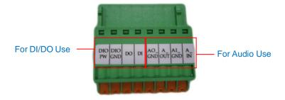
To connect audio devices, map the pins to one of the pin combinations below:
