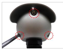
NOTE: A cable is connected inside the camera; do not abruptly pull the back cover.
