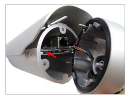
3. When done, ensure the rubber seal is aligned and attached to the back cover and then close the back cover by tightening the three (3) screws.
