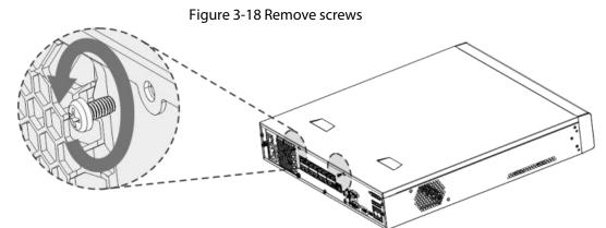
Step 2 Remove the case cover along the direction shown in the following arrow.
