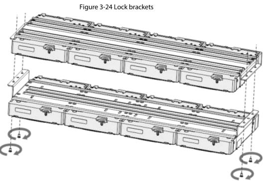
Step 7 Place the bracket to the device and then fasten the screws on the sides of the bracket.
