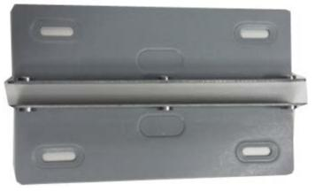
Step 3 Fix the CD-ROM bracket at the HDD bracket.
