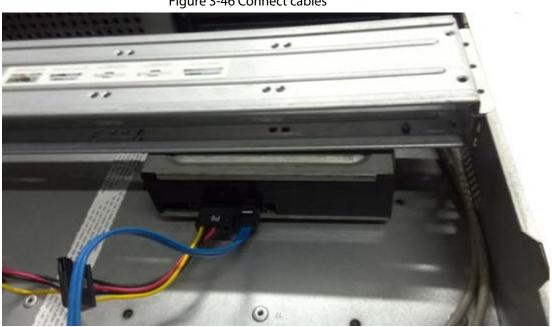
Figure 3-46 Connect cables
