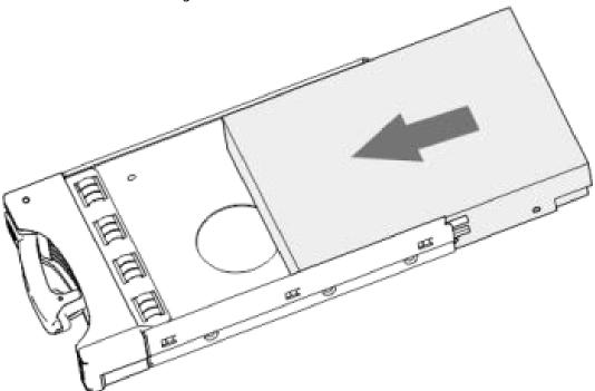
Step 3 Fasten the screws on the sides of the HDD box.
