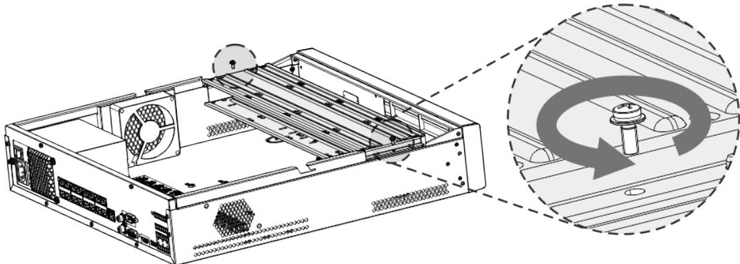
**Step 4** Match the four screw holes on the HDD with the four holes on the bracket and then fasten the screws.
