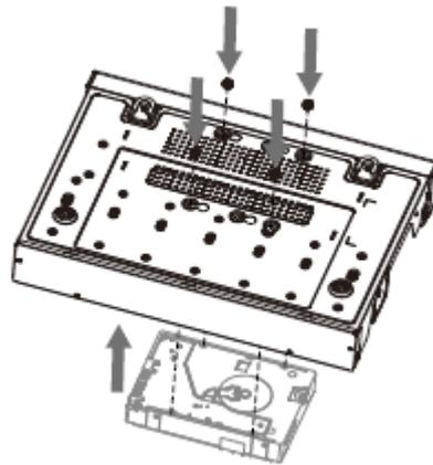
Step 4 Connect HDD to the device using data cable and power cable.
