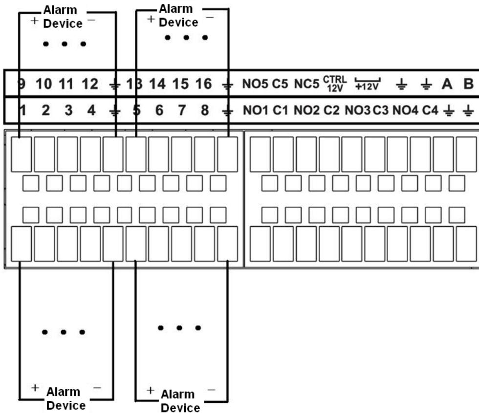
Figure 2-83 Alarm input port
