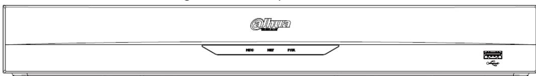
The NVR22-8P-I/NVR22-8P-I2 front panel is shown as below.
