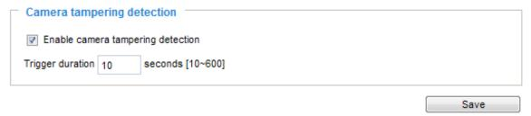
Please follow the steps below to set up the camera tamper detection function:
