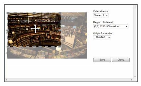
Click **Viewing Window** to open the viewing region settings page. On this page, you can configure the Region of Interest and the Output Frame Size for different streams. For example, you can crop only a portion of the image that is of your interest, and thus save the bandwidth needed to transmit the video stream. As the picture shown below, the area of your interest in a parking lot should the vehicles. The blue sky is of little value for the surveillance purpose.
