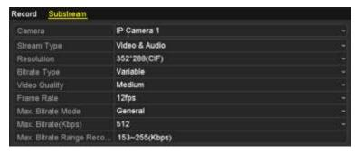
Figure 5. 4 Sub-stream Parameters
