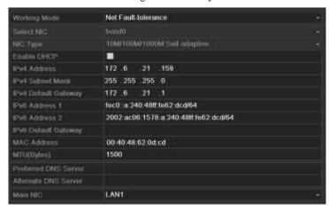
Figure 9. 2 Net Fault-tolerance Working Mode
