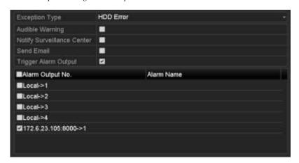
Figure 10. 23 Configure HDD Error Alarm
