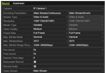
Figure 5. 3 Recording Parameters
