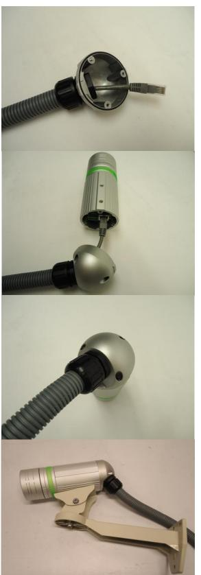
8. Tighten the domed sealing nut.
